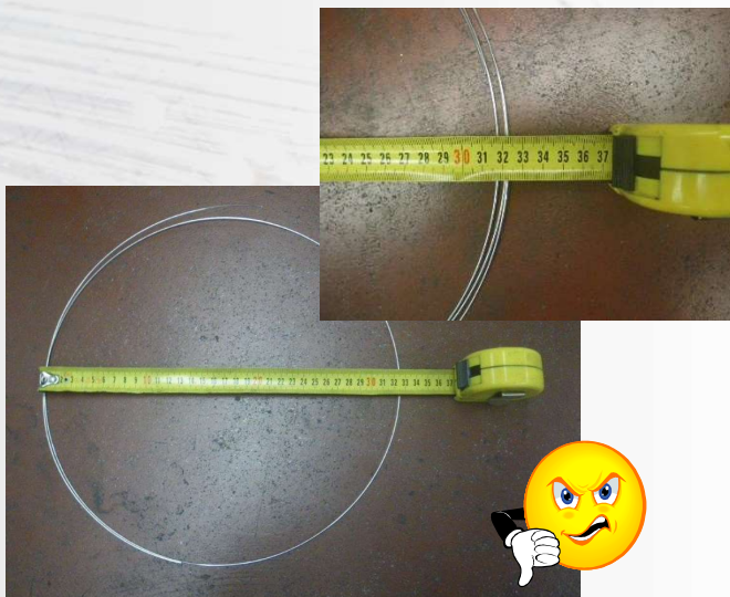
Competitor ER 5356 1.2 mm, Cast \varnothing 320 mm
