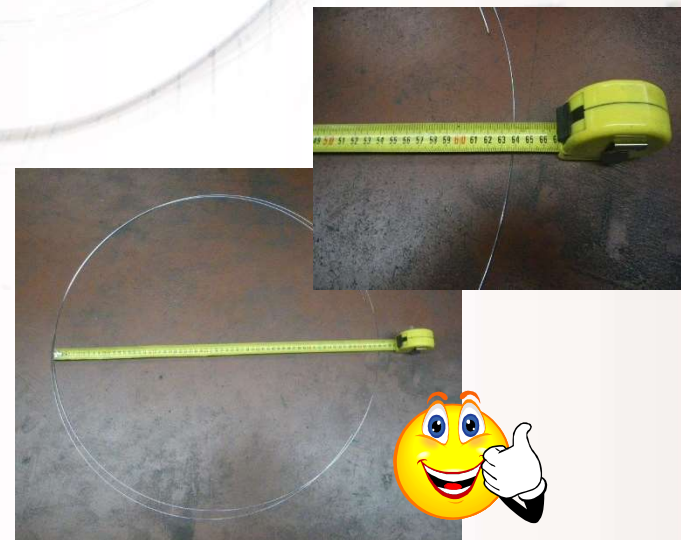
Safra ER5356 1.2 mm, Cast \varnothing > 640 - 800 mm
