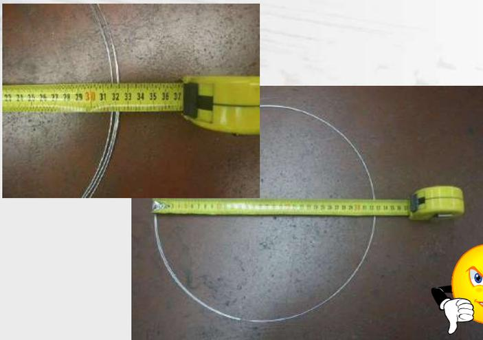
Competitor ER 5356 1.2 mm, Cast  $\varnothing$  320 mm
