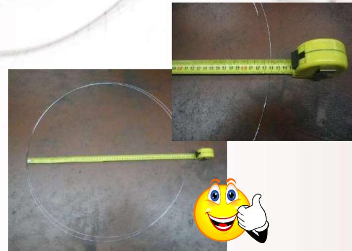
Safra ER5356 1.2 mm, Cast  $\varnothing$  > 640 - 800 mm
