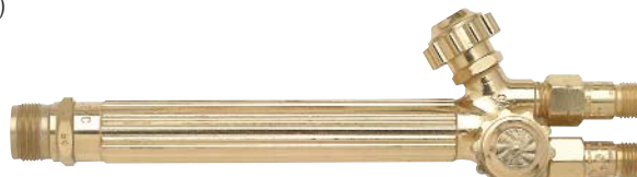
Model V-315C Length: 9 1/2"; Weight: 1.4 lbs. Cuts 6", welds to 1" (page 9)
